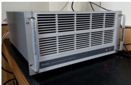
Battery test station
