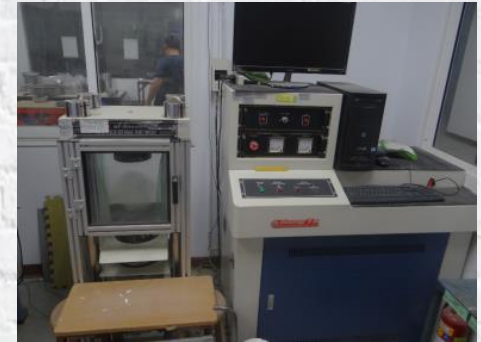
Concrete compressive strength machine
