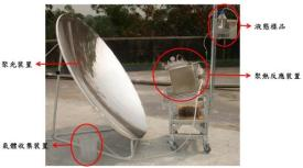
Solar heat for pyrolysis of biomass.
